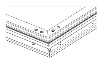
7.Fold over the screen material and secure each notch of it lining up with one snap lung on the frame. First work toward each corner and then toward others.
