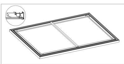
8.Install all 4 thin panels into each frames, make sure the bevels of the thin panels and frames are coincided and the flatness of the screen material during all procedures.
