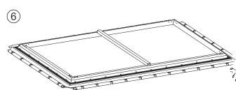
6.Place the assembled frame onto the screen material and ensure the frame is placed on the middle of the screen material.
