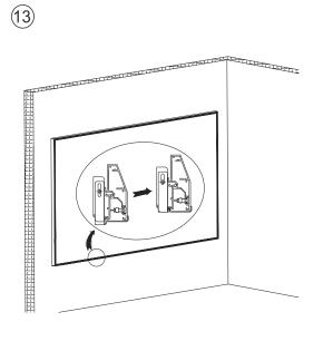
13.Lock the screen into the lower mounting brackets and fasten the screws. Installation completed.
