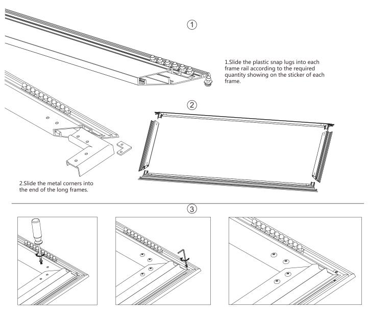
3.Put all the frames together and screw in 4 corner screws into each corner of the frame.
