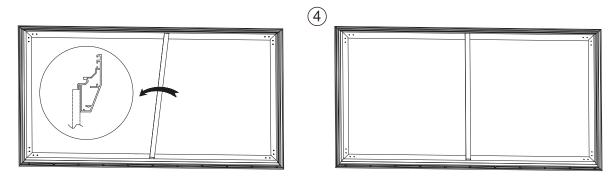
4.Install the support bar in the proper place. (Quantity of the support bars is up to the screen size)
