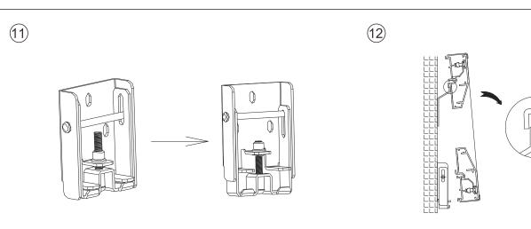
11.Loosen the screw of each lower mounting bracket.
