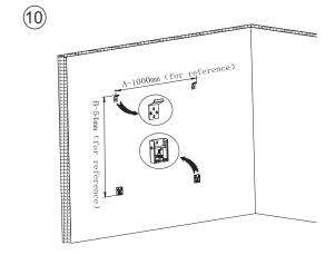
9. Measure the frame the distance for A and B showing as above.
