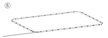
5.Make sure the floor is clean, keep the viewing side facing down and unroll the screen material. Use the appropriate rods for each side, insert the rods into the pockets on the edges of the screen.
